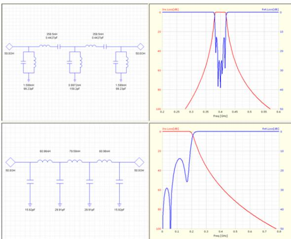
Fig. 5. Filters for the RF ports.
