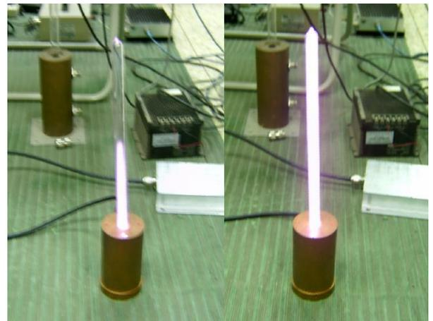
Fig. 7. Reconfiguration test of plasma antenna prototype.
