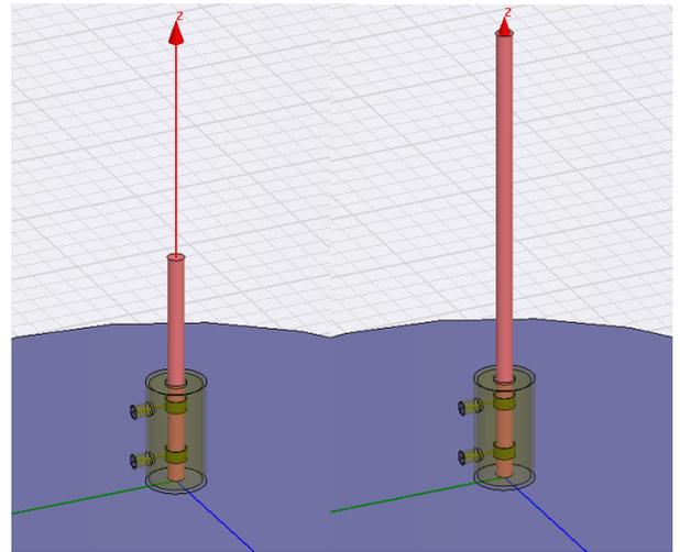
Fig. 6. Reconfigurable length of plasma antenna.
